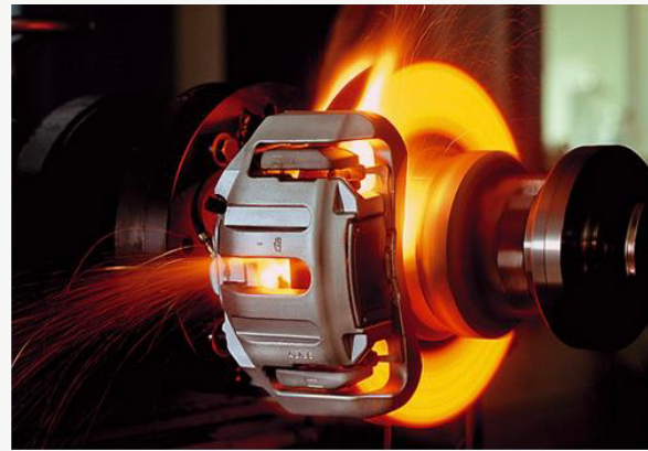
FIGURE 2: Red-hot brake rotor on a test stand
