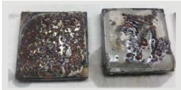
FIGURE 9: Corrosion on grey cast and FNC after 20 hours
