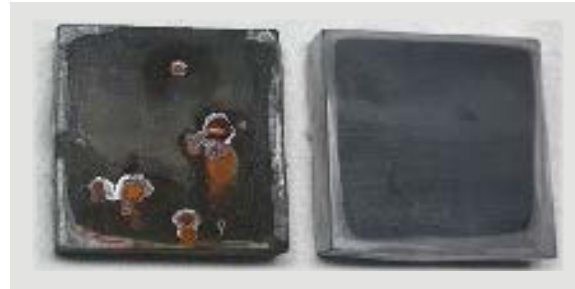
FIGURE 10: Corrosion on ONC and smart ONC after 100 hours
